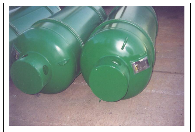
850 I. AMMONIA NH 3 TEST PRESSURE 33 bar
