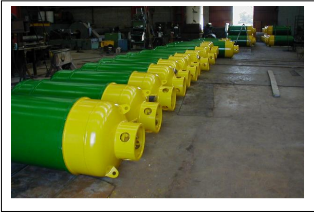
850 I. SULPHUR DIOXIDE SO 2 TEST PRESSURE 33 bar
