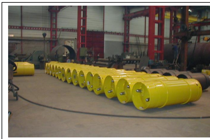
930 I. CHLORINE Cl2 TEST PRESSURE 43 bar
