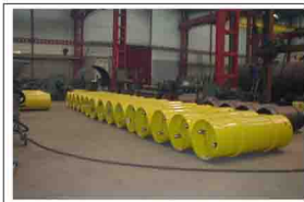
930 L. CHLORINE Cl2 TEST PRESSURE 43 bar
