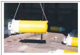
400 I. CHLORINE CL2 TEST PRESSURE 33 bar
