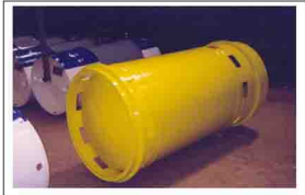
990 I. HYDROGEN CHLORIDE TEST PRESSURE 120 bar
