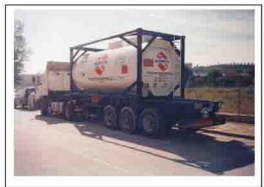
21,670m 3 SO2 ISOCONTAINER 20' TEST PRES.13,4 bar
