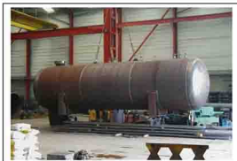
50 m 3 . NH3 LIQUIFIED SERVICE PRESSURE 22 bar
