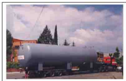
125 m 3 CO2 LIQUIFIED SERVICE PRESSURE 23 bar
