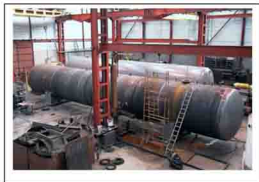
165 m 3 . CO2 LIQUIFIED SERVICE PRESSURE 23 bar
